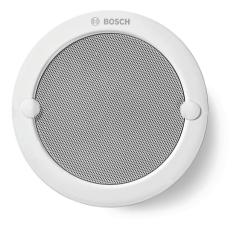
This A/B Ceiling loudspeaker with fire-dome has two independent 6 W loudspeaker systems and is suitable for sound systems where redundancy is requested. In normal situations, both loudspeakers are powered with the same audio signal from independent amplifiers. In case the A-line fails, the other connected loudspeaker receives the signal from line B and the other way around.
