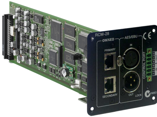
Figure 6.15: OMNEO device with two separate IP connectors; on the pictured device the connectors are labeled Primary and Secondary, on other devices these connectors may not be labeled.
