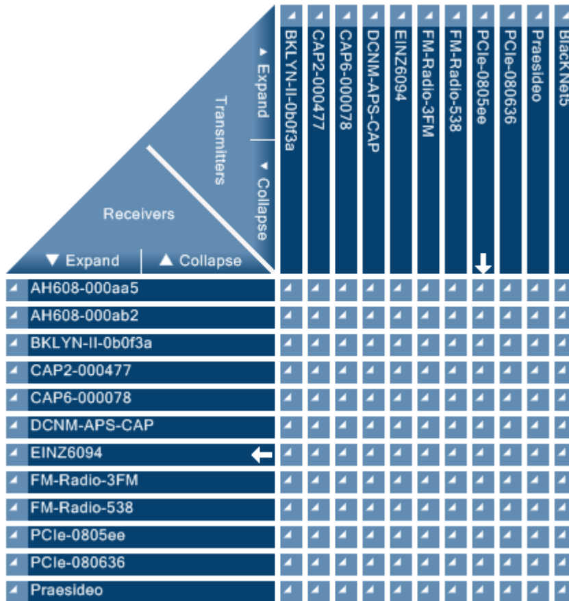
Figure 5.4: Example of OMNEO Control production environment; notice the BlackNet5 device that has transmit channels only (see also figure 6.5).
